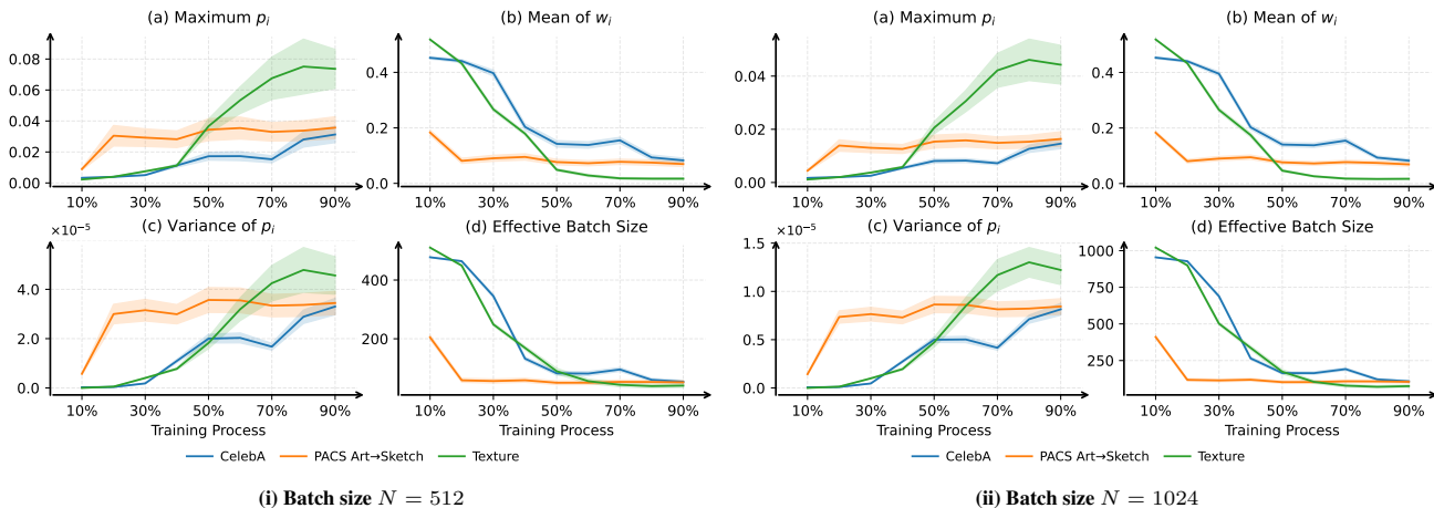
Figure 4. Training dynamics under batch sizes 512 and 1024: (a) the mean unnormalized weight \hat{\mathbb{E}}[w_i] = S/N , which decreases over time, (b) the maximum normalized weight \max_i p_i , which increases but to a lower ceiling for N = 1024 (c) the variance \text{Var}(p_i) , which increases to a lower ceiling for N = 1024 , and (d) the effective batch size B_{\text{eff}} = (\sum_i p_i^2)^{-1} , which is larger for N = 1024 . Colors indicate datasets. Shaded regions show mean \pm std across independent batches.
